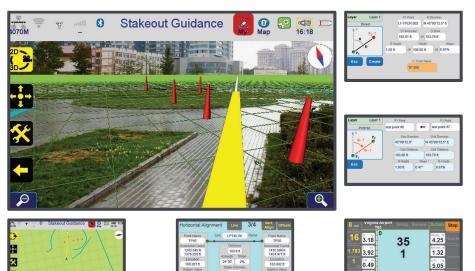
With Visual Stakeout (VSO) the virtual location of the point to be staked can be seen by a "flag" shown on the Triumph-VS camera image. This visual aid helps to navigate quickly to the point and makes stakeout jobs fast and fun. Use VSO as an easy and convenient way to get close to the target point, and then switch to the regular stakeout mode to perform precise measurement.
